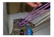
Continue to feed the Dyneema control line back up to the double block, feeding the line from front to back.
