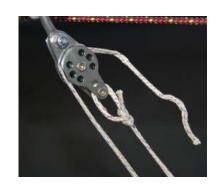
6 Take the V12 back up to the top block and feed it through from the bottom.
