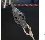
2 Tie the length of Vectran V12 (1.45 m) in a bowline loop through the top block.
