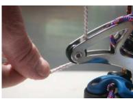
Thread the V12, previously attached 5 to the top block, through the pulley/becket from the top.
