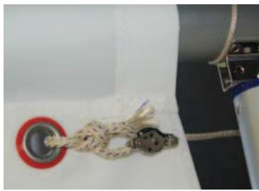
1 Tie the **block and becket** to the **6 mm Vectran x 1.2 m** (part 6) length and feed it through the Cunningham eye of the sail from the starboard side.
