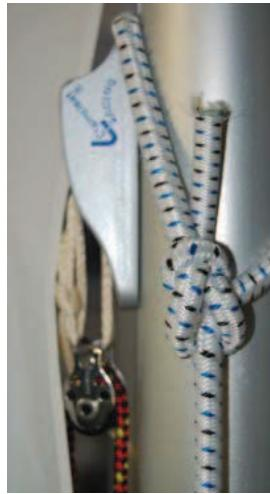
**26** The clew hook can be used as an alternative method of securing the clew of the sail. This may require pliers to open the eye slightly to fit the **micro block** (Part 9).
