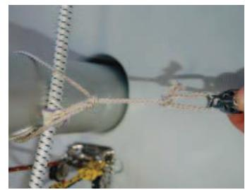
3 Tie the air block to the mast below the boom vang tang with the piece of 3 mm Vectran (part 10).
