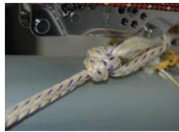
2 Tie a bowline around the boom vang tang with the vang in place.
